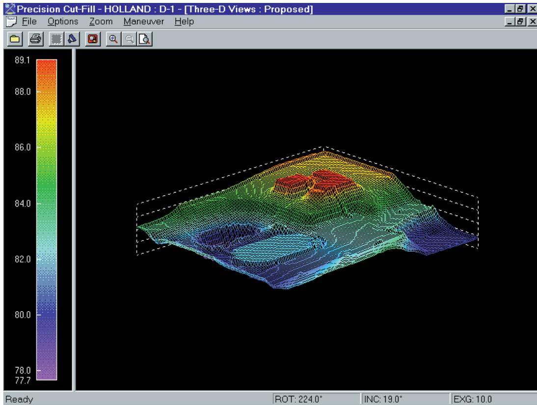
*Cut & Fill quantities are quickly determined and 3-D graphics displayed for immediate analysis.*
